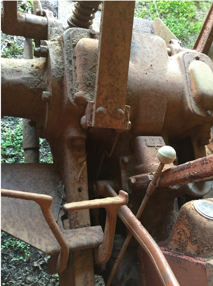
Rear transmission case and dual clutch system of Andalusia’s Allis-Chalmers WD, showing the four forward gears and reverse gears in the operator’s console, as well as the seat and the feet bars.
