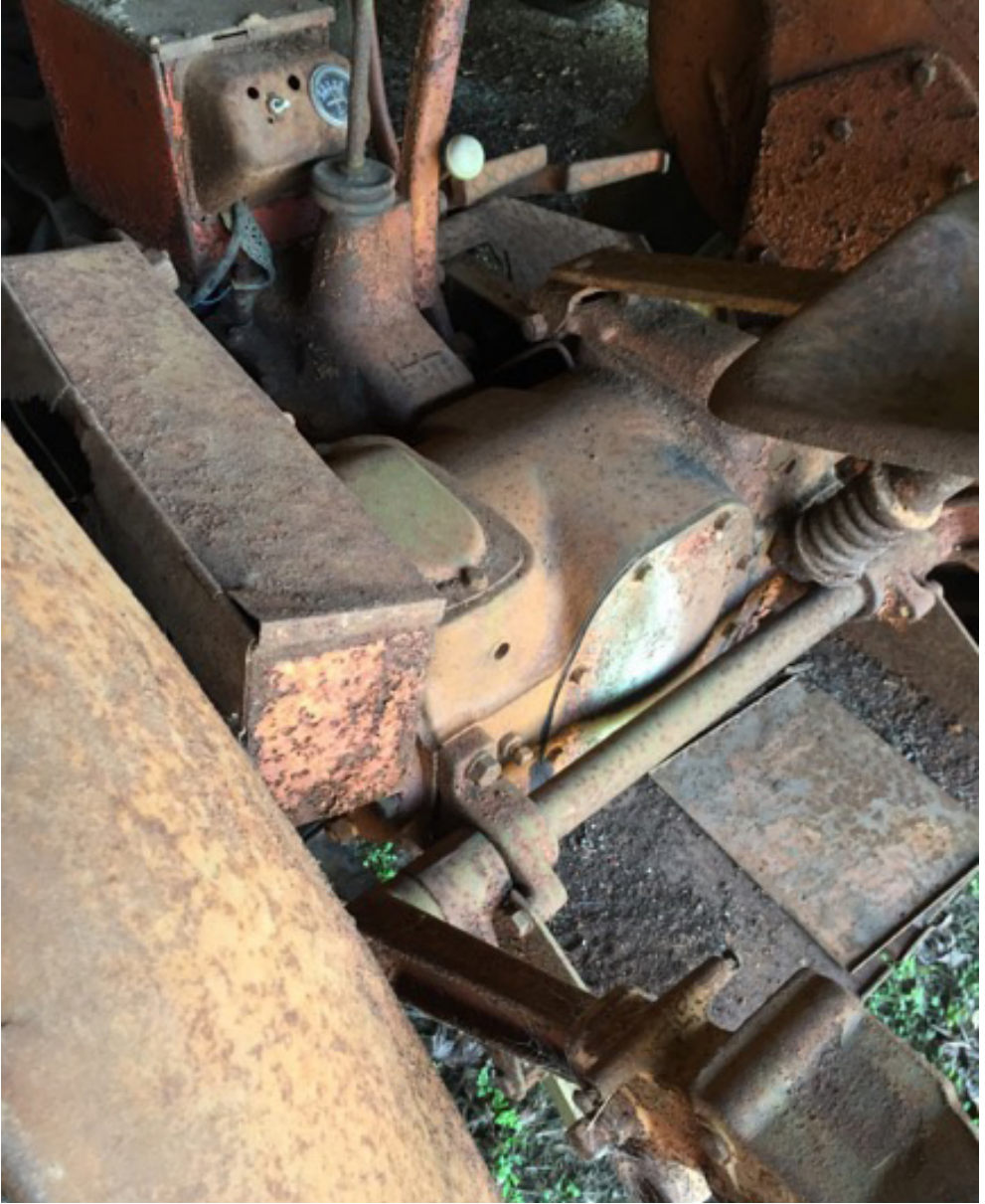
Allis-Chalmers model WD equipped with a two-clutch power control. The dual clutch featured a foot-operated dry clutch capable of disconnecting the PTO driveline from the engine. A hand-operated wet clutch permitted PTO operation when the tractor was stopped.
