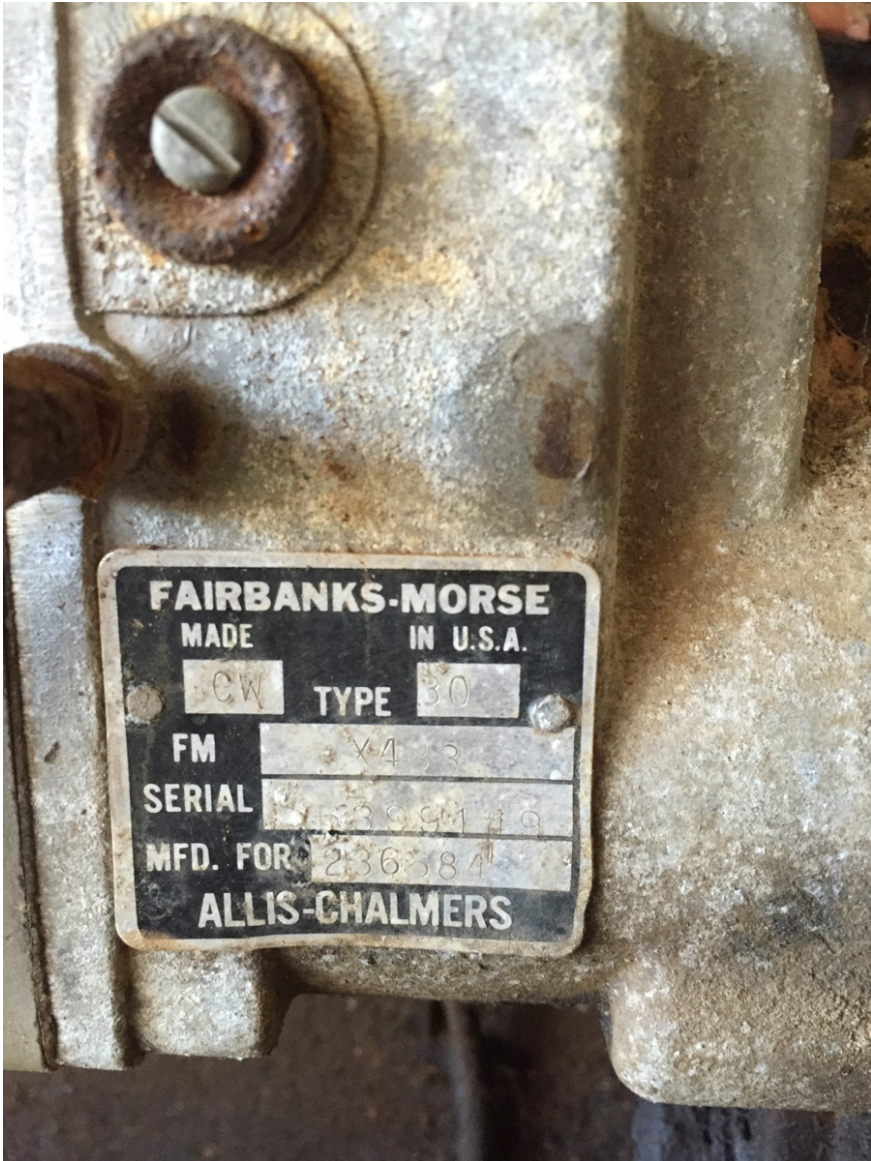
Rebuildable magneto from Andalusia's model WD Allis-Chalmers. The magneto sends the spark to fire the Allis-Chalmers's engine.
